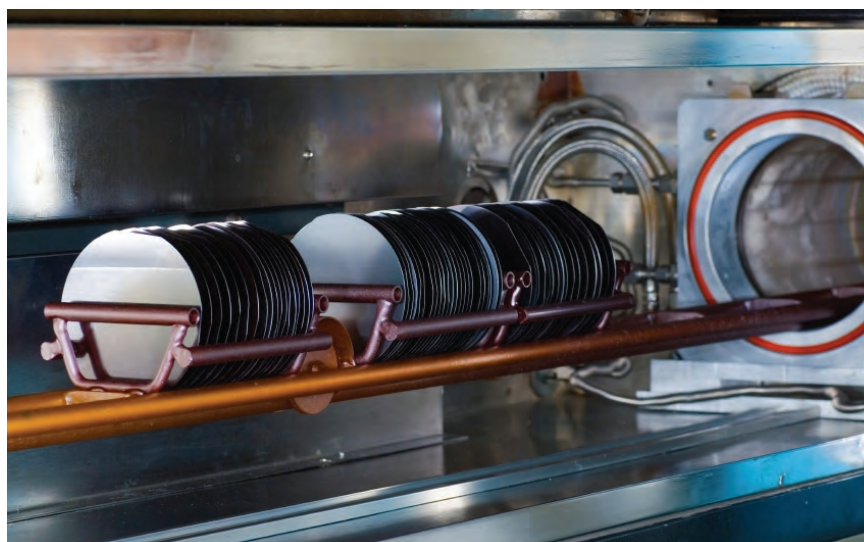
Wafers pictured in front of furnace tube entrance.
