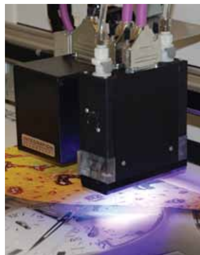
UV-LEDs are compact and have low voltage, making them an ideal source for applications where the UV source is attached to a moving carriage such as inkjet systems.
