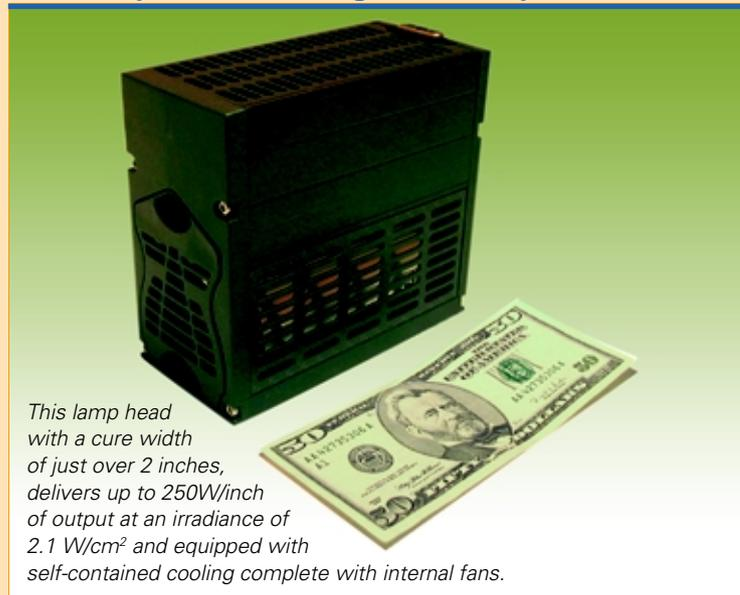
*This lamp head with a cure width of just over 2 inches, delivers up to 250W/inch of output at an irradiance of 2.1 W/cm<sup>2</sup> and equipped with self-contained cooling complete with internal fans.*
