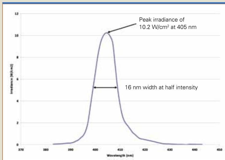
the integrating sphere and close the door. The die is powered and the UV energy is released from the LED over its entire viewing angle. The emitted UV bounces around inside the sphere and the energy that is radiated onto a detector of known area and located somewhere on the
