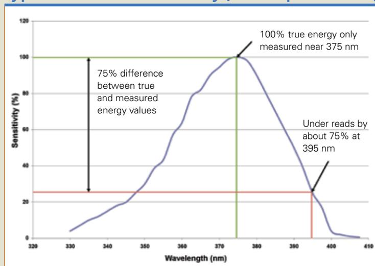
physics behind an integrating sphere or how the irradiance is exactly calculated. What you should take away, however, is an appreciation of the complexities involved in accurately measuring UV-LED irradiance and how integrating spheres, due to their shape and size, aren't practical measuring tools for most commercial UV-LED applications.
