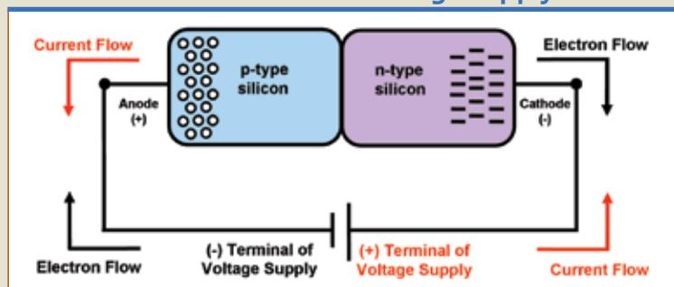
flow from the positive terminal of the voltage supply through the n-side, across the depletion zone and through the p-side to the negative terminal of the supply. Zener or avalanche diodes are based on this scenario.
