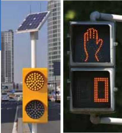
High-brightness LED traffic signal (left) and crossing signal (right).
