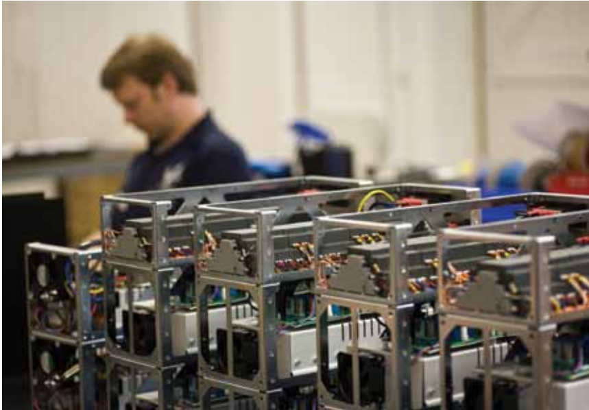
Power supplies being assembled for a UV system.
