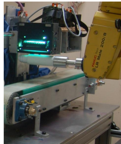
Digital inks are cured almost instantly by UV lamps supplied by Integration Technology, Ltd.
